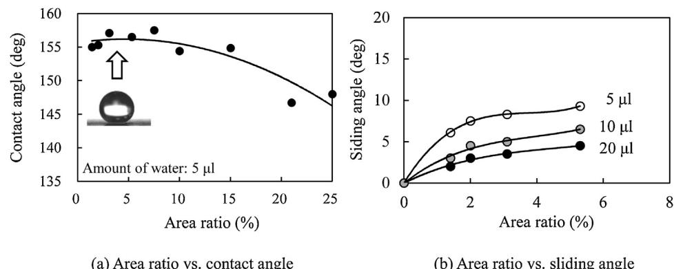
**Fig. 5.** Relationships between area ratio and static contact angle (a) and between area ratio and sliding angle (b).
