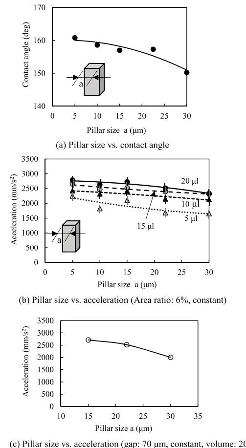
**Fig. 8.** Relationship between pillar size and static contact angle (a), and relationship between pillar size and acceleration ((b) and (c)). The area ratio was set to be constant at 6 % in (b) (the pillar gap was in the range of 20 to 90  $\mu\text{m}$ ). The pillar gap was set to be constant at 70  $\mu\text{m}$  in (c) (the area ratio was in the range of 3 to 6 %).
