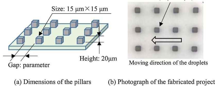
**Fig. 2.** Dimensions of micro pillars.
