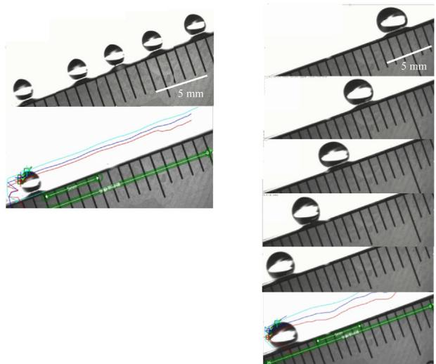
(d) Moving behaviors of the droplets ( $5 \mu\text{l}$  (left) and  $20 \mu\text{l}$  (right)), area ratio: 5.3%
