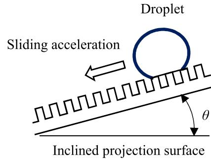
**Fig. 1.** Improvement of transporting a small droplet by decreasing density of the projection formed on the inclined surface.
