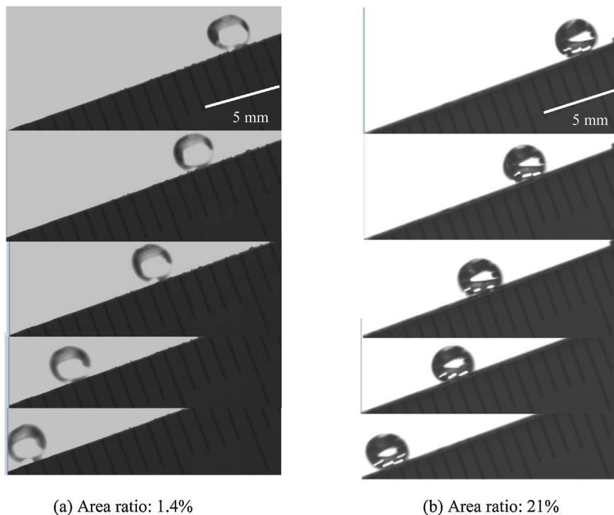
**Fig. 9.** Behaviors of droplets (10  $\mu\text{l}$ ) in the case of the different area ratios (1.4 and 21%, sliding length: about 20 mm, 1000 fps).
