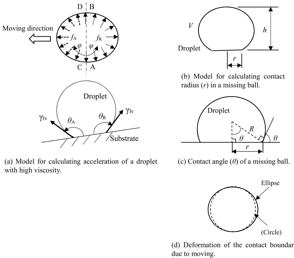
**Fig. 15.** Model to calculate the resisting force acting on the contact boundary of the droplet (a) and the model for calculating the contact radius and the contact angle by using a missing ball (b) and (c), respectively.
