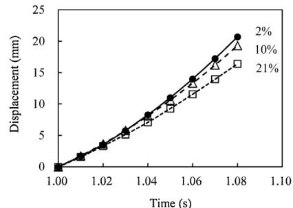
(a) Displacement ( $10 \mu\text{l}$ , Inclination:  $20^\circ$ , Area ratio: 2, 10, and 21 %)
