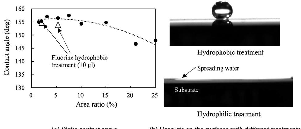
**Fig. 11.** Relationships between area ratio and contact angle when hydrophobic treatment was conducted (a). Droplet was not formed on the surface with hydrophilic treatment (b): water spread on the surface.
