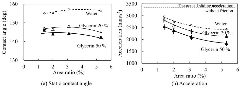
Fig. 12. Relationship between area ratio and static contact angle (a) and acceleration (b) when viscosity of liquid was varied (droplet: 10  $\mu\text{l}$ ).
