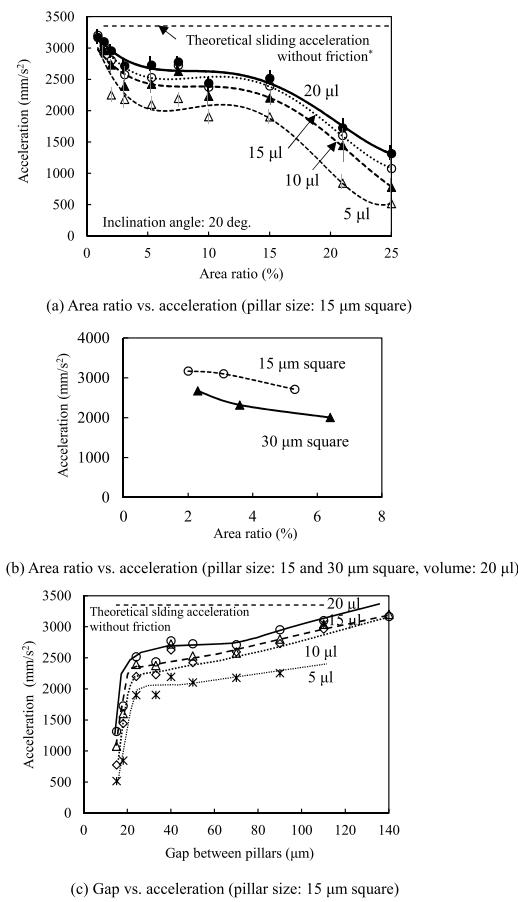
**Fig. 7.** Relationships between area ratio and acceleration. Pillar size: 15  $\mu\text{m}$  square (a) and 15 and 30  $\mu\text{m}$  square (b). Figure (c) shows the relationship between the gap and the acceleration, where the area ratio of (a) is changed to the gap. (Inclination angle: 20 deg. Sliding acceleration without friction is 3350  $\text{mm}/\text{s}^2$ .)
