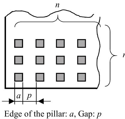
**Fig. 3.** Definition of area ratio. The area ratio was calculated from the pillar size and the gap:  $(n^2 \times a^2) / (n \times a + (n-1) \times p)^2$ , where  $a$ : edge length of the pillar,  $p$ : gap between the pillars, and  $n$ : number of the pillars in the row or the column.
