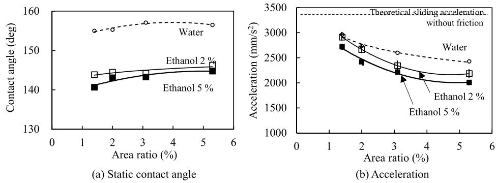
**Fig. 13.** Relationship between area ratio and static contact angle (a) and acceleration (b) when surface tension of liquid was varied (droplet: 10  $\mu\text{l}$ ).
