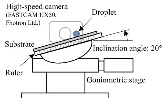
**Fig. 4.** Measurement apparatus used in this work.
