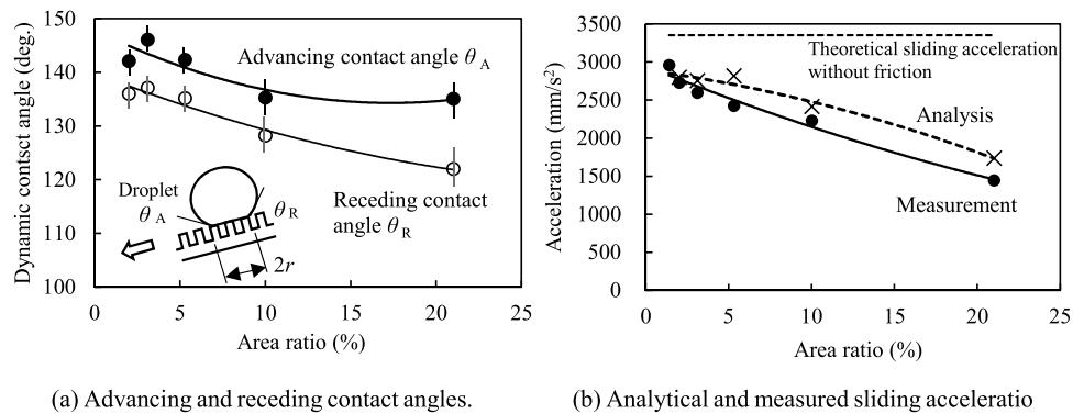
**Fig. 10.** Measured dynamic contact angles (a) and sliding accelerations by calculation using dynamic contact angle and contact radius (b) (droplet: 10  $\mu\text{l}$ ).
