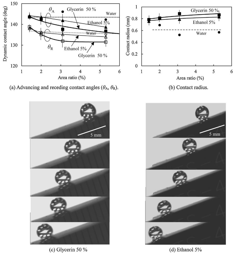
**Fig. 14.** Relationships between area ratio and dynamic contact angle (a) and contact radius (b) of liquid with different viscosity and surface tension (droplet: 10  $\mu\text{l}$ ). Moving behaviors of droplets (c) and (d).
